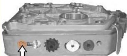
1995 & 1996 01M's use a plastic end plug.
