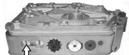
1997 & Up 01M's use an aluminum end plug.
