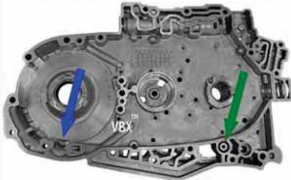
Early Style With TCC Blow Off Ball
